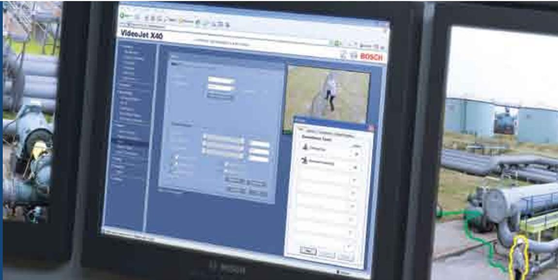
Any events detected by the system that fit the pre-defined criteria are depicted clearly on-screen. Object outlines, color-coded according to the alarm status, overlay the monitor images to show their position. Factors such as aspect ratio and perspective are automatically accounted for.
