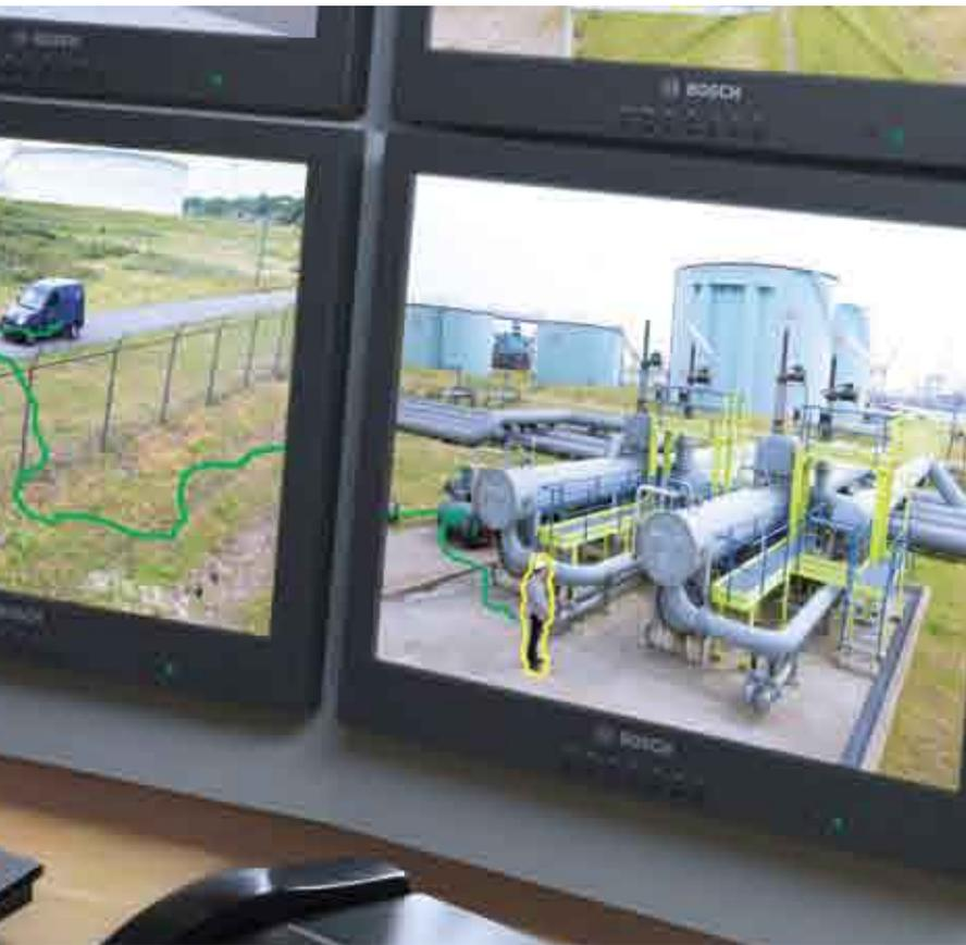
Working independently on each camera, Bosch IVA operates without a central analytics server. You can choose a wide variety of advanced detection functions, ranging from idle object to trajectory tracking. Live images are analyzed instantly and the resulting data stream accompanies the video feed.
